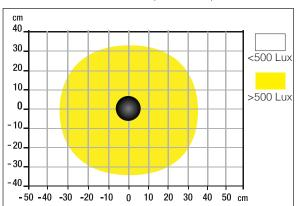
Measurement of Lux on the worktop with a 40 cm profile:
