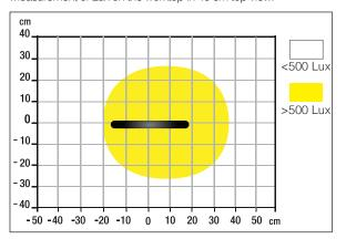
Measurement of Lux on the worktop with a 40 cm profile:
