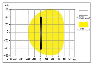
Measurement of Lux on the worktop with a 50 cm profile:
