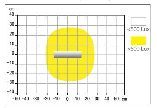
Measurement of Lux on the worktop with a 35 cm profile:
