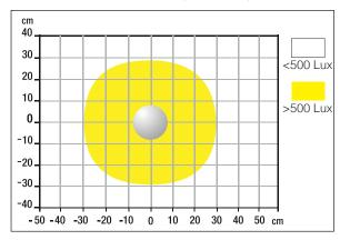
Measurement of LUX on the worktop with a 35 cm profile:
